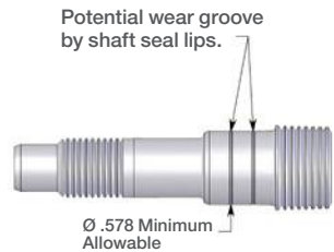
SC125 001.2 Shaft, Outlet Wear
